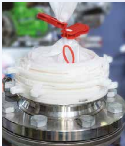
Separation of the SafePortBag using the SafeSeal System
